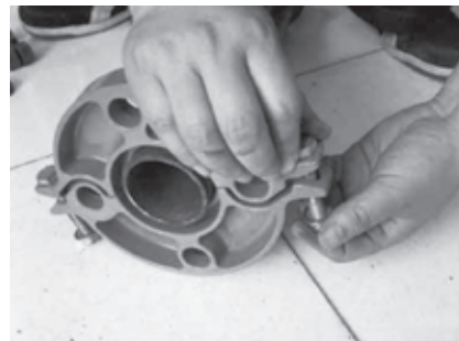
3.Put another part of flange in the groove, screw the bolts and nuts averagely on the two parts
