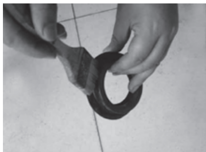
4.Check the gasket to keep the availability in any situation, spread lubricant on surface of gasket.
