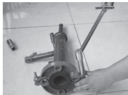
6.Secure the bolts and refer to Table 5 for Bolt-Torque.
